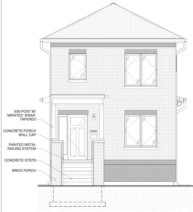
① FLAT ROOF - ELEVATION 1/4" = 1'-0"
